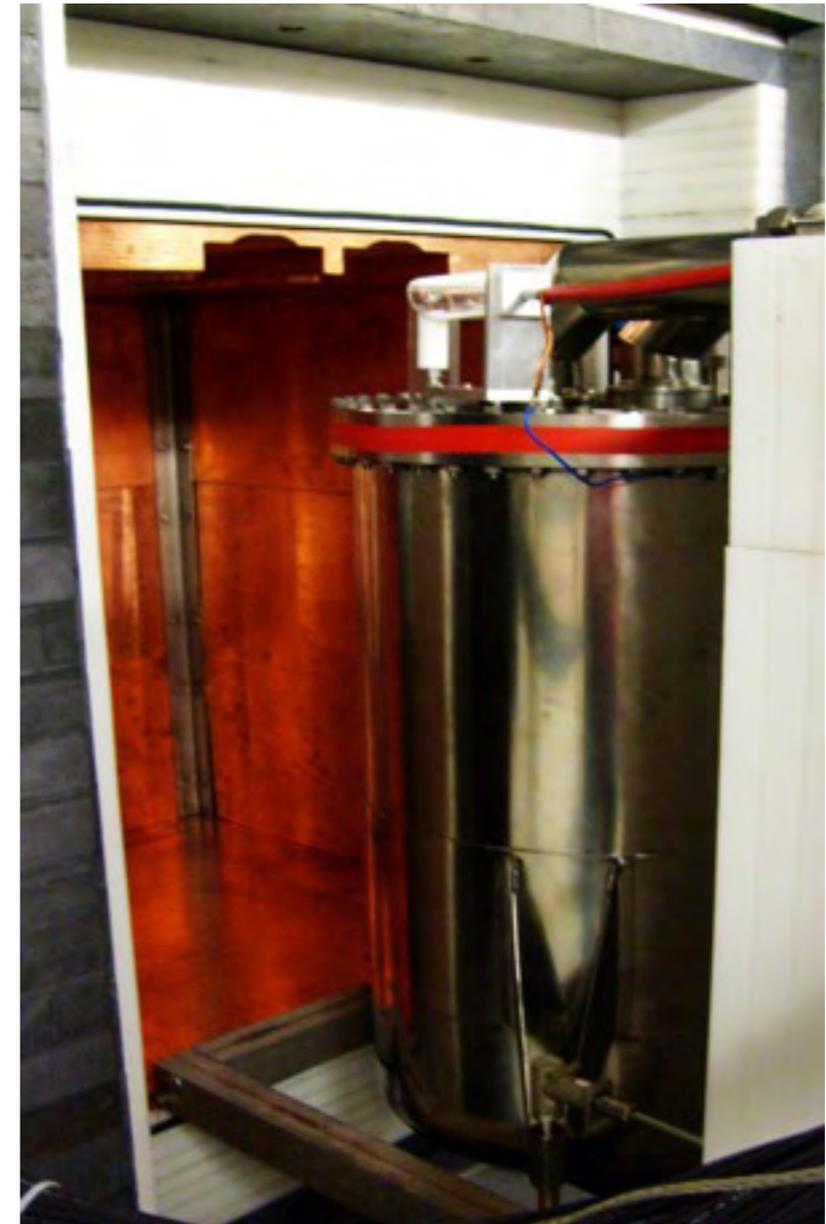
The XENON100 detector in its low-background shield at LNGS
